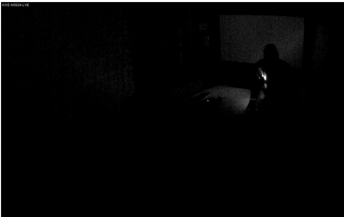
The above images from AXIS M3024-LVE—depicting the same scenario of a man with a small flashlight in a dark room—show the difference that IR illumination makes for surveillance in the dark. The image at left is without the use of IR illuminators. The image at right uses IR light from the camera's built-in IR LEDs. IR light is invisible to the human eye but visible to the camera.
