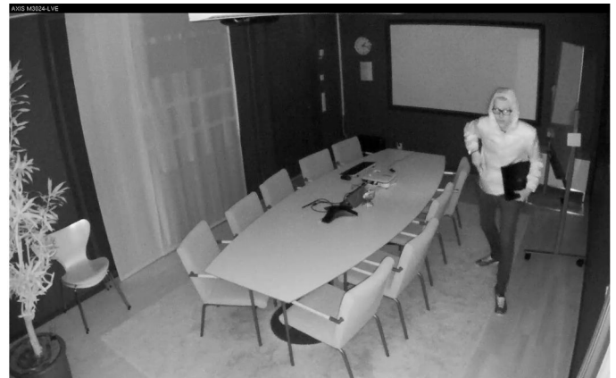
The above images from AXIS M3024-LVE—depicting the same scenario of a man with a small flashlight in a dark room—show the difference that IR illumination makes for surveillance in the dark. The image at left is without the use of IR illuminators. The image at right uses IR light from the camera's built-in IR LEDs. IR light is invisible to the human eye but visible to the camera.
